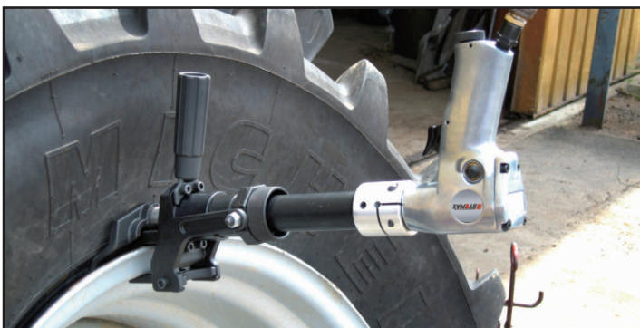
► Operation of Bead Breaker
