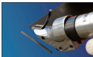
► Operation of Air Metal Shear
