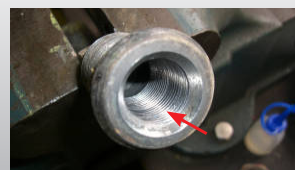
• Rust & Dirt on the Inner Thread
