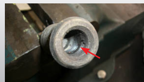
• Rust & Dirt on the Inner Thread
