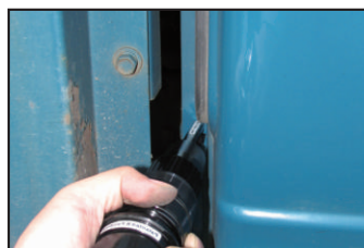
► Operation of Spot Drill
